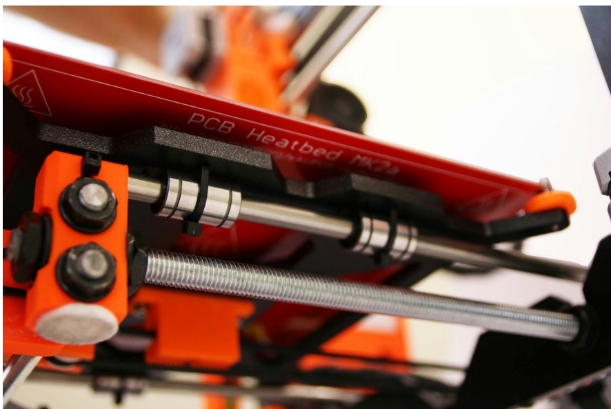
Pict. 23 - Properly tightened zipties under the heatbed
