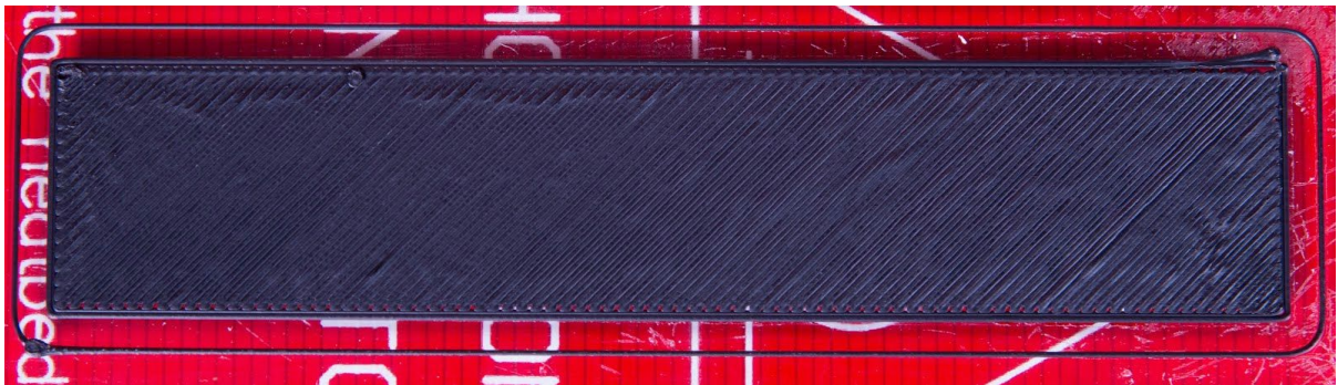
Pict. 6b - Calibrated printer shows continuous filament layers.
